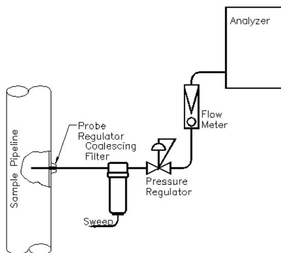
Figure 7: Typical Sample Conditioning System
