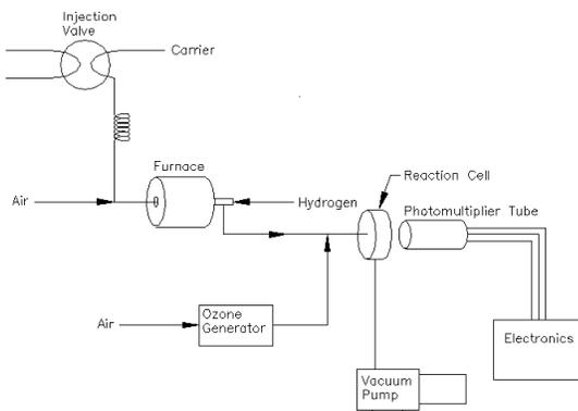
Figure 2: Sulfur Chemiluminescence Analyzer
