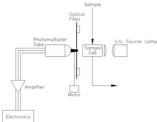
Figure 4: Ultraviolet Absorption Analyzer
