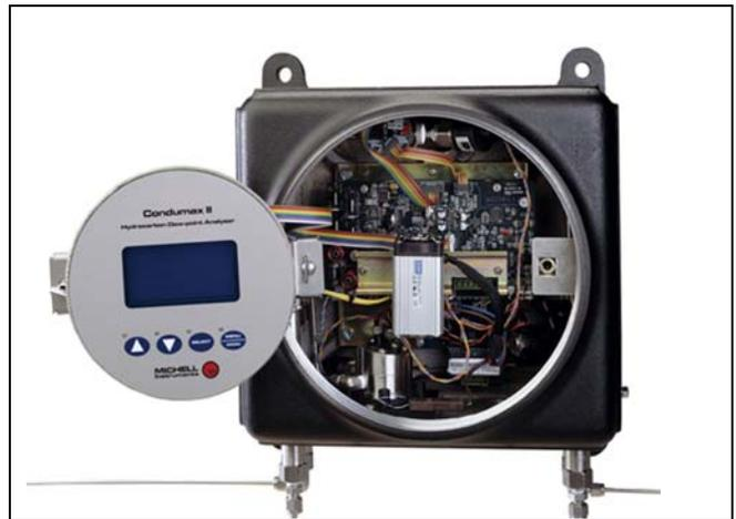
Figure 6. CONDUMAX II Main Unit: Internal view
