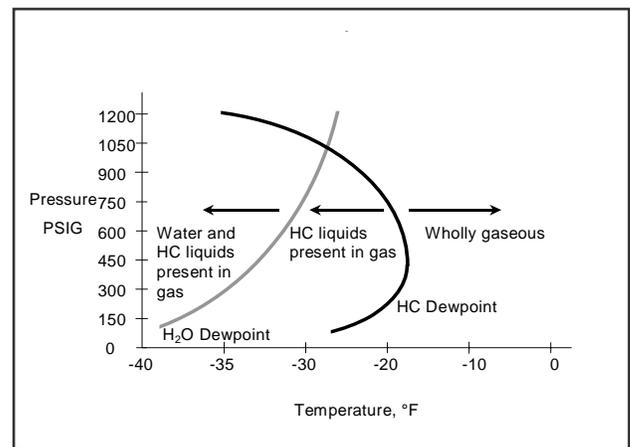
Figure 1. Typical retrograde phase envelope for natural gas
