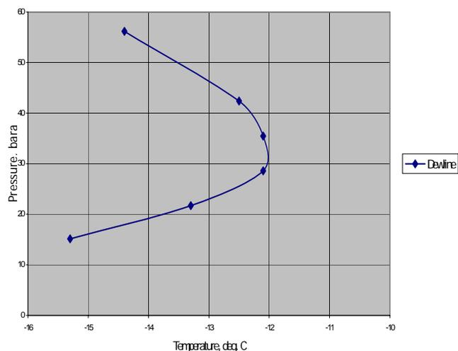
Figure 10. Example of phase envelope produced by CONDUMAX
