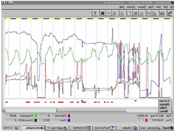
The flow computer performs its calculations every second, based on live values, and accrues the volume and MMBTU; however, the editor must recalculate based on hourly averages. For this reason, the data manager's recalculation routines should employ some type of skewing technique to more closely approximate what the flow computer would have calculated had the error not existed in the original data.
