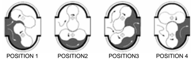
**FIGURE 1. ROOTS Rotary Positive Displacement Operating Principle**
