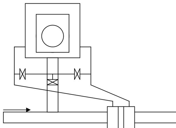
**Figure 1. Schematic of the Basic Components of an Orifice Meter Chart Recorder Installation**
