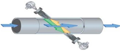
Figure 1: Ultrasonic Transit Time Principle
