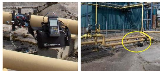
Figure 6: Clamp-on flow meter on natural gas at 100-psig inside large manufacturing plant
