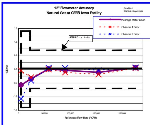
Figure 5: Calibration results of 2-path meter at CEESI
