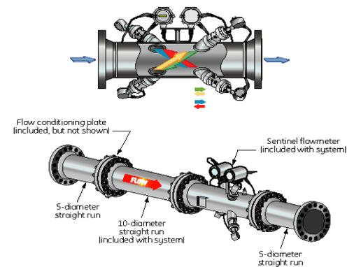
Figure 4: Sentinel 2-Path Meter shown with complete meter run
