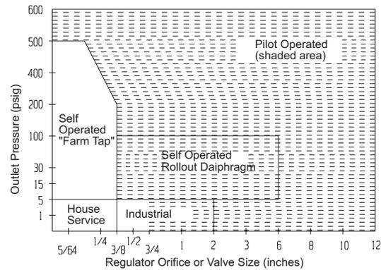
valve sizes, a Pilot Operated Regulator generally offers better accuracy and more capacity at a lower cost. Refer to the Regulator Selection Chart of Outlet Pressure versus Orifice Valve Size (Figure 2) for a graphic indication of where Self Operated Regulators are used in the gas industry.
