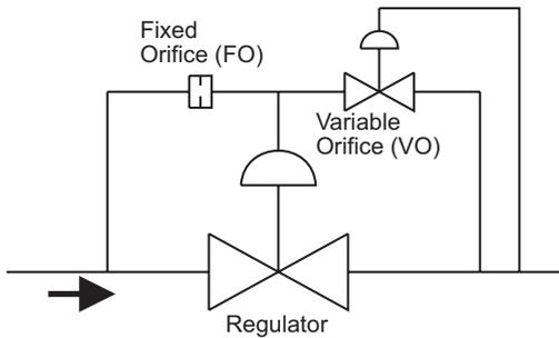
**Fig. 3 Typical Pilot System**
