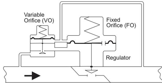
**Fig. 5 Loading Type Pilot Operated Regulator**
