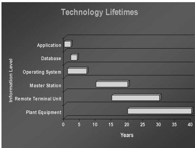
**FIGURE 2. Technology Lifetimes in SCADA**
