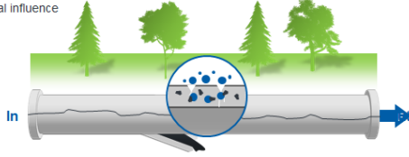
Figure 3: Causes of Pipeline Leaks
