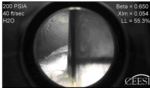
FIGURE 4. Stratified Flow Through an Orifice Plate
