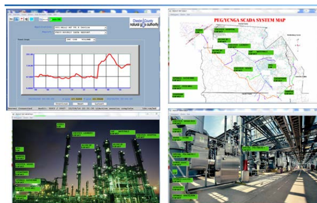
Figure 4. Facility / Plant GUI Example
