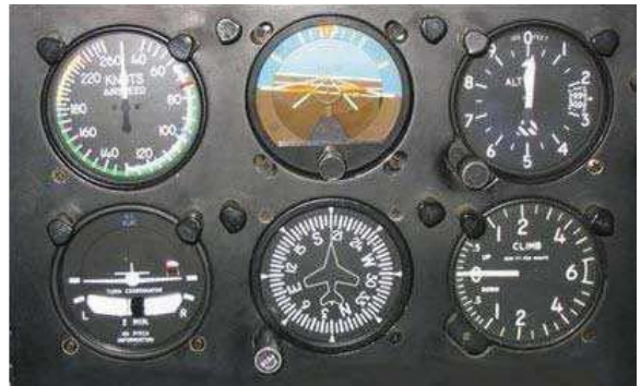
Figure 3. Sacred six instruments in cockpit
