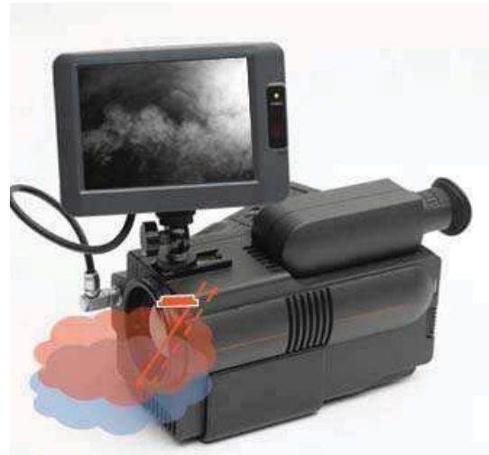
Figure 5: Video Image of Gas Leak
