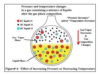
It can therefore be stated that *when liquid is present* in a natural gas sample, a change in either the temperature and/or the pressure will result in a change of the gas phase composition.
