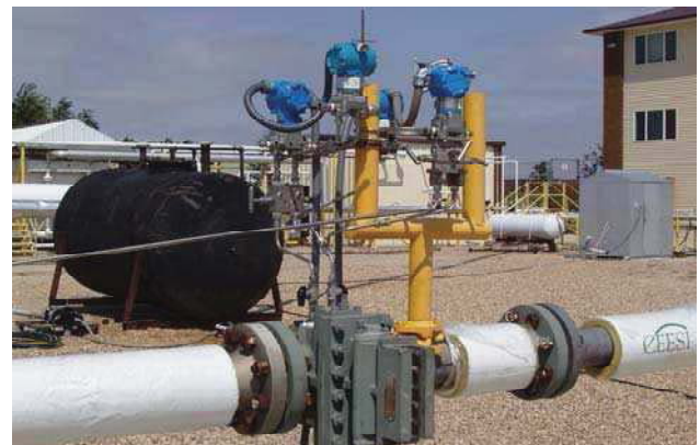
Figure 6. 4", orifice meter under wet gas flow testing.
