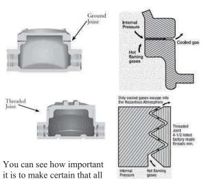
flame paths are protected during installation and maintenance, and even during handling, shipping, and storage of explosion-proof material. Even slight damage to a flame path can permit burning gases to escape, igniting the surrounding atmosphere. Also, all cover bolts must be installed for the same reason. A single missing bolt could allow the release of flaming gases.
