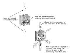
Sealing fittings are designed to be filled with a chemical compound after the wires have been pulled. As the compound hardens, it seals passageways for
