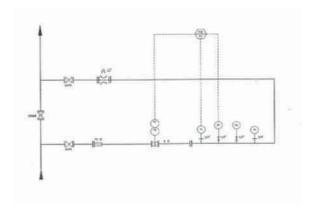
There are two ways to install a Master Meter on an existing Field Meter skid. One way is to use a three-valve manifold downstream of the existing meter run shown in the P&ID above. Downstream of the field meter is the preferred location because the flow profile into the Field Meter is not disturbed.
