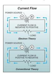
The ampere (A) is the term used to refer to electrical current moving in an electrical circuit. Electrical current is the movement of negatively charged particles called electrons within the circuit. By definition, one ampere is the equivalent of  $6.241 \times 10^{18}$  electrons per second when
