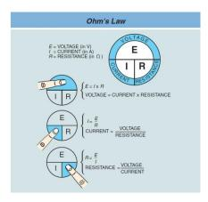
Ohm's Law is the most important and most often applied law in electricity and in electrical maintenance work. To understand electricity and work in electronics you must thoroughly understand Ohm's Law and know how to apply it effectively in solving electrical problems.
