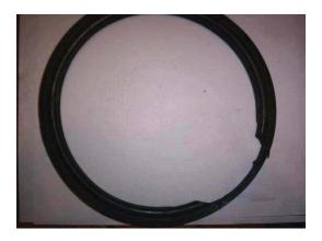
Other problems occur when flange gaskets protrude into the meter tube; the error can be either a positive or negative in nature. It is important to make sure that the proper size and ANSI rated flange gasket is used in the meter tube. The picture below illustrates the effect of the wrong size gasket upstream of the orifice plate. Note the deflection of gas, as evidenced by the shaded area of the tube and plate.
