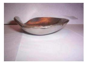
In extreme situations, the orifice plate can be blown completely out of the orifice plate carrier. It is not uncommon for hydrates to form in the winter months. If the vane "pin" is weak or damaged, the velocity of the gas flow may cause the hydrate to move and hit the vanes. Once the pinning device is compromised, the vanes will move downstream with the flow.
