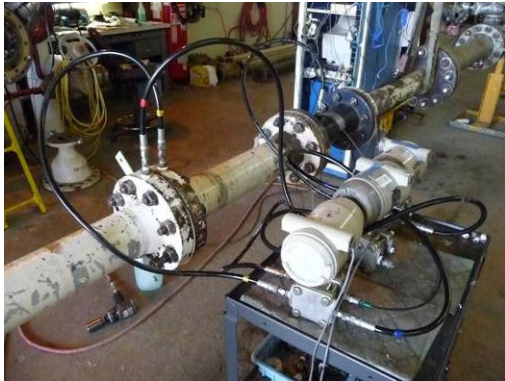
Fig 5. Flange installed plate with air flow.
