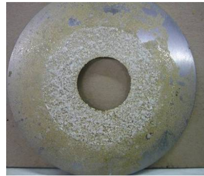
Fig 21. A heavily contaminated orifice plate.
