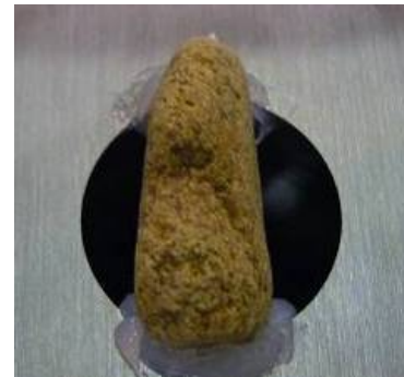
Fig 29. Rock trapped at an orifice plate.
