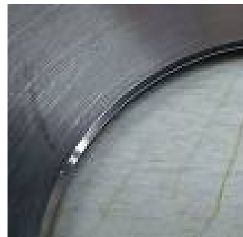
Fig 18. Chamfered (0.02") orifice edge.
