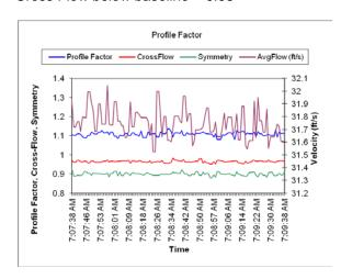
This could indicate a blockage upstream of the meter.
