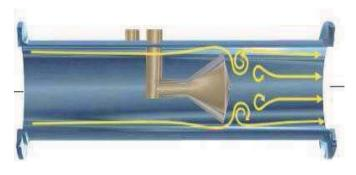
The centrally located cone inside the meter body reshapes the profile of the flow as it enters the meter body. The cone can have many different diameters which makes most "Cone Meters" a fixed Beta Ratio. The principle of the meter is similar to that of the Orifice Meter and the Venturi Meter, using a Beta Ratio. As the flow comes into contact with the cone, it creates a low pressure region just downstream of the cone. See illustrations below:
