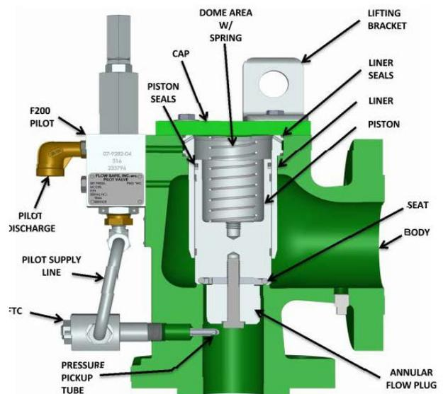
7. High-Performance Spring Style: Potential (compressed) energy of a spring determines set point. 95% bubble tight on plastic seat, 98% bubble tight on O-ring seat, full lift at set point (0 overpressure), adjustable blowdown from 3% to 20%.
