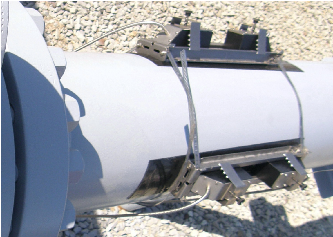
Figure V. – TRANSDUCERS MOUNTED ON PIPE IN REFLECT MODE
