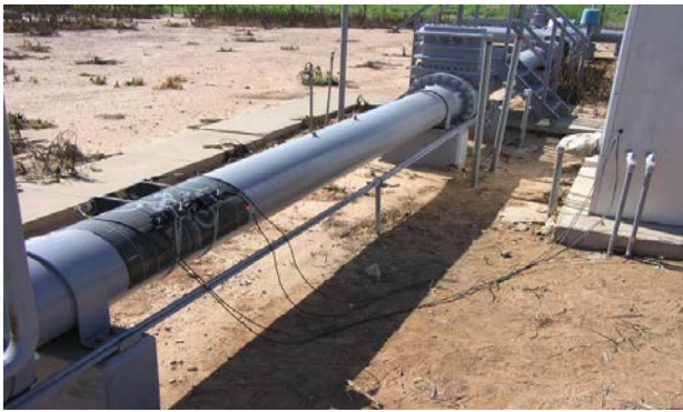
Figure IX.-Clamp-on Compared to Orifice Meter
