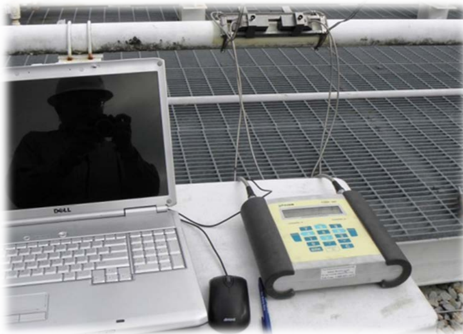
Figure IV. - CLAMP-ON METER INSTALLED ON PIPE
