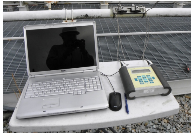
Figure XIV. - CLAMP-ON DETECTION OF LEAK
