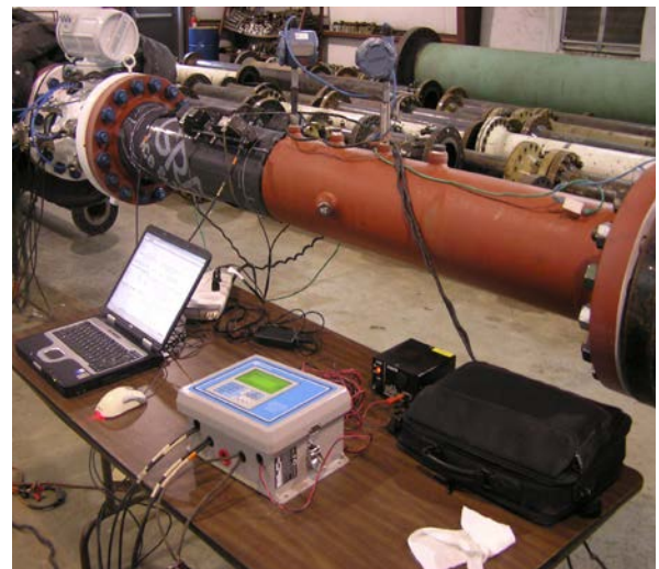
Figure XV. - CLAMP-ON REFERENCE AT CUSTODY METER CALIBRATION
